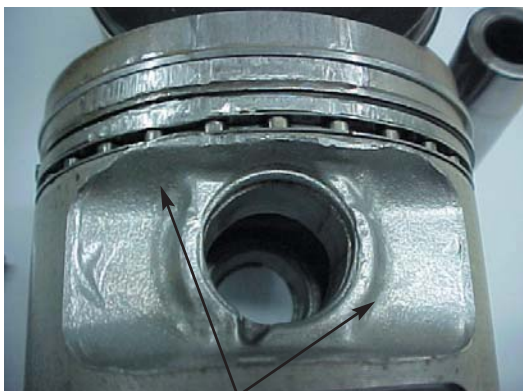
Fig. 1.1.1 Damages caused by circlip
