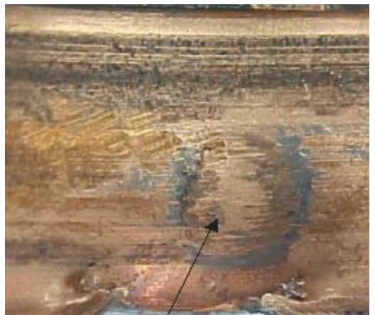
Fig. 10.2.5 Internal mark formed by odd material
