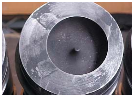
Fig. 2.6.5 Irregular spraying done by the nozzle
