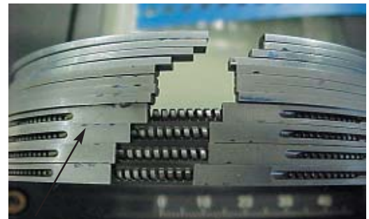
Fig. 3.5.7 Considerable wear on the third groove
