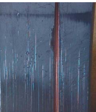
Fig. 8.2.5 Enlarged photo of a channel opened by an odd solid material, strange to the bearing
