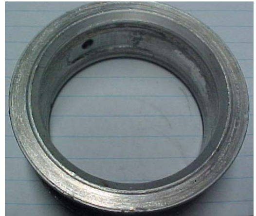
Fig. 8.1.2 Totally worn-out flange
