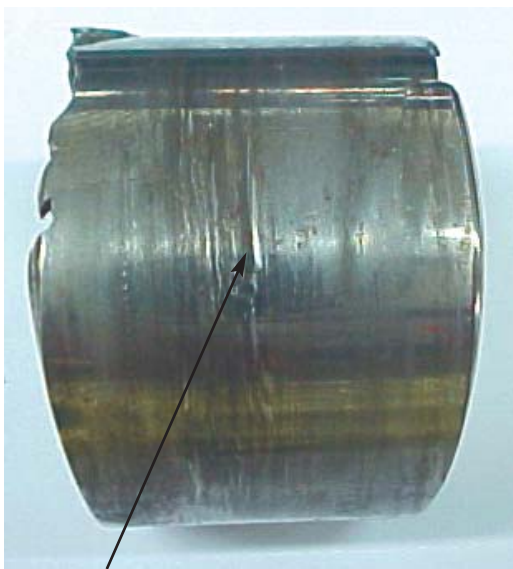
Fig. 10.3.1 Incorrect bushing mounting mark
