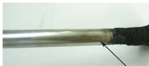
Fig. 11.1.4 Scuffing due to insufficient clearance between valve and valve guide
