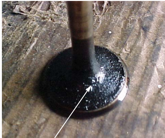
Fig. 11.9.3 Contaminated inlet valve with lubricating oil crust due to excessive clearance between valve and valve guide or malfunction of oil seal
