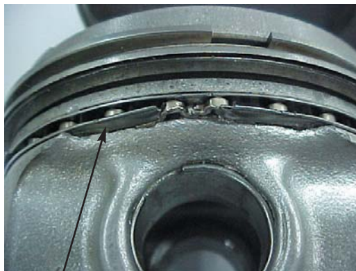
Fig. 1.1.2 Damages caused by circlip
