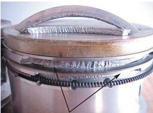
Fig. 2.15 Broken lands in piston (Otto-cycle engine)
