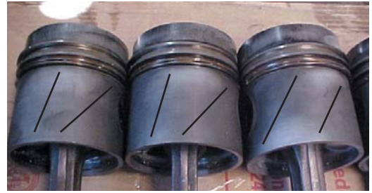
Fig. 1.3.1 Inclined marks at the piston skirt region
