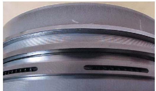
Fig. 3.5.6 Worn-out piston ring of the third groove
