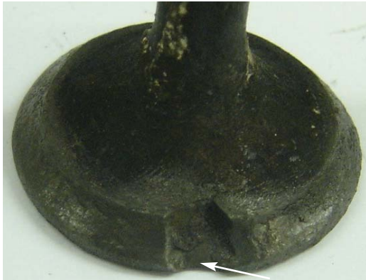
Fig. 11.8.1 Localized disintegration at the seat region
