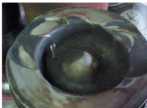
Fig. 2.6.4 Irregular spraying done by the nozzle
