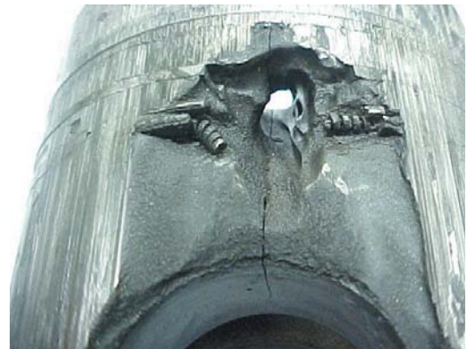
Fig. 2.7.11 Destruction of the crown and the pin boss region, due to irregular function of injection nozzle
