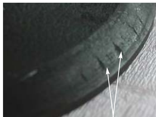
Fig. 11.5.2 Fissures on the valve seat
