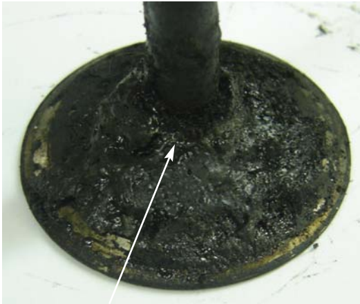
Fig. 11.9.3 Contaminated inlet valve with lubricating oil crust due to excessive clearance between valve and valve guide or malfunction of oil seal
