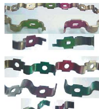
Fig. 3.7.2.9 Form and colors in new expanders (without rework)
