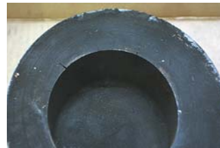
Fig. 2.13.6 Cracks at combustion bowl rim
