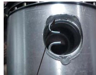
Fig. 1.1.3 Damages caused by circlip
