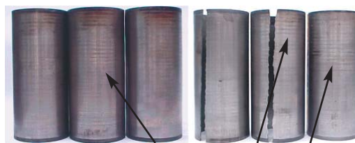
Fig. 5.2 cylinder liners with machining marks from engine block
