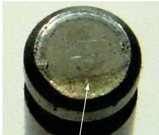
Fig. 11.9.4 Marks indicating that the valve hasn't rotated. Rocker arm deficiency
