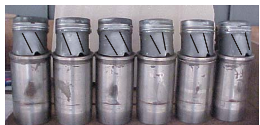
Fig. 1.3.4 Inclined marks at the piston skirt region
