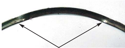
Fig. 3.4.1 Ring was twisted during mounting
