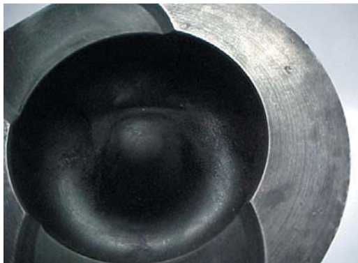
Fig. 2.13.1 Machining marks at piston crown
