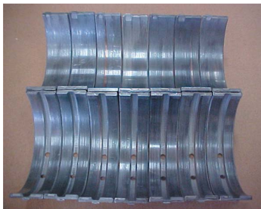
Fig. 8.2.4 Contaminated main bearings with circumferential scratches
