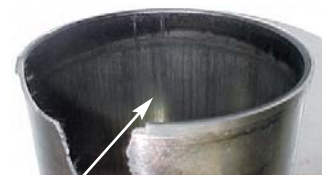
Fig. 6.3 Wear and scratches formed by solid particle admission into the cylinder
