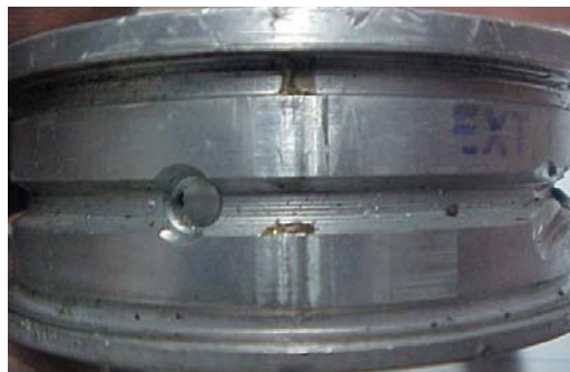
Fig. 8.13 Glue/adhesive on bearing's external lubrication channel
