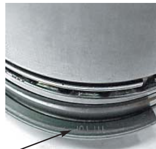
Fig. 3.1.1 Piston ring mark mounted towards the lower side
