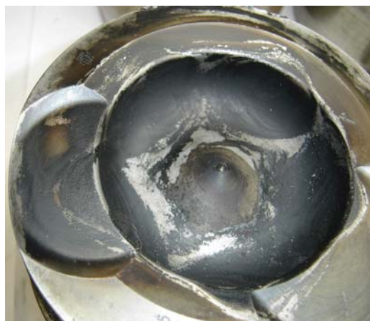
Fig. 2.6.3 Irregular spraying done by the nozzle
