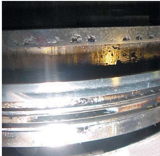
Fig. 3.6.5 Flaking-off of the piston ring coating
