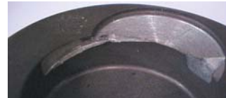
Fig. 2.13.5 Machined valve recess
