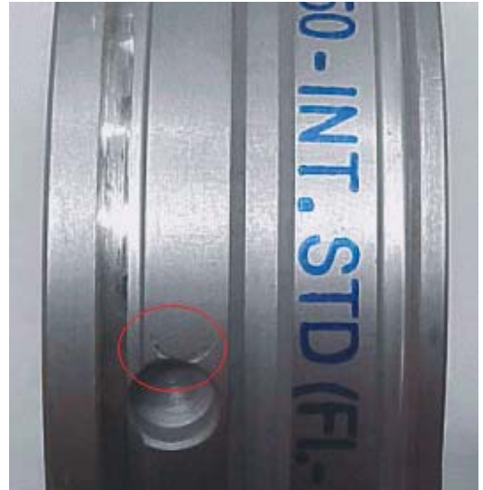
Fig. 8.13.1 Pin mark on external bearing side
