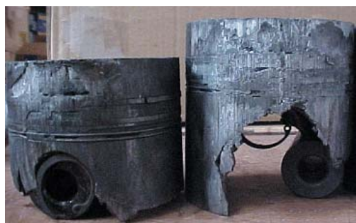
Fig. 2.6.7 Scuffing started at the top land, followed by rupture at the pin boss
