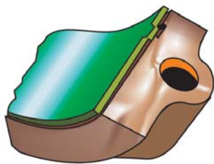
Fig. 9.4 Interference between the bearing lug the housing lug
