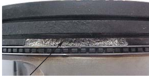
Fig. 2.15.1 Broken land in piston (Otto-cycle engine)
