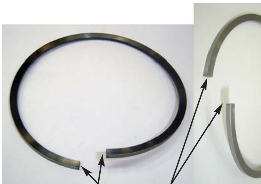
Fig. 3.4 Displaced butts due to incorrect mounting
