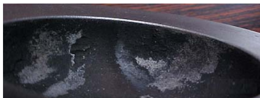
Fig. 2.6.2 Spraying occurs partially out of the combustion chamber
