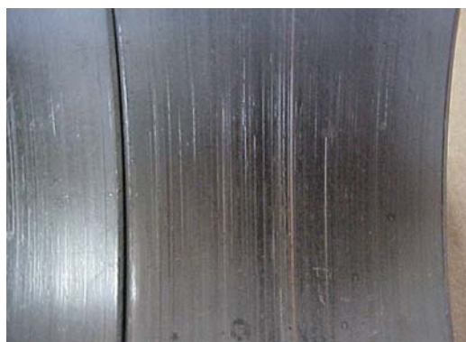
Fig. 8.2.6 Contaminated con rod bearing with circumferential scratches
