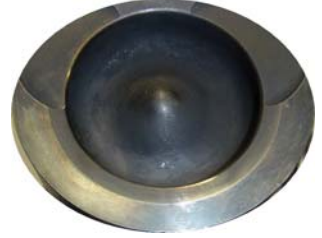
Fig. 2.13.4 Machined valve recess
