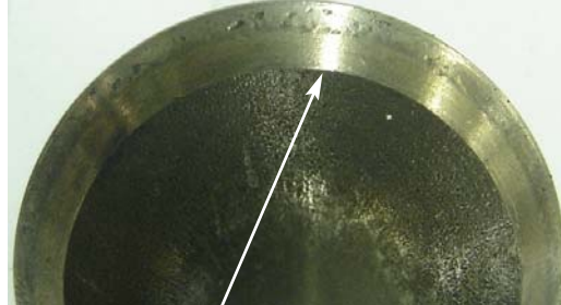
Fig. 11.7.2 Wear at the valve head region
