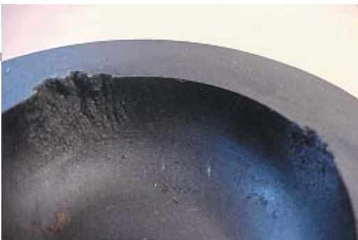
Fig. 2.7.1 Partial destruction of the combustion chamber
