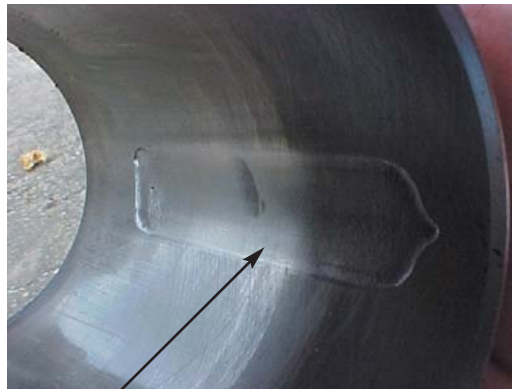
Fig. 6.2.1 Mark originated by the piston pin displacement after the circlip expulsion
