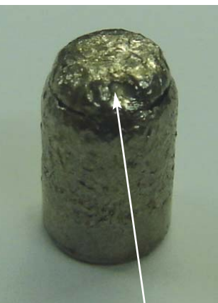
Fig. 11.4.1 Breakage at the keeper groove region
