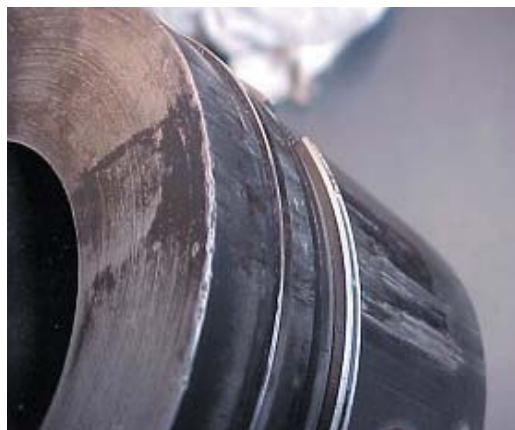
Fig. 2.6.6 Irregular spraying done by the nozzle
